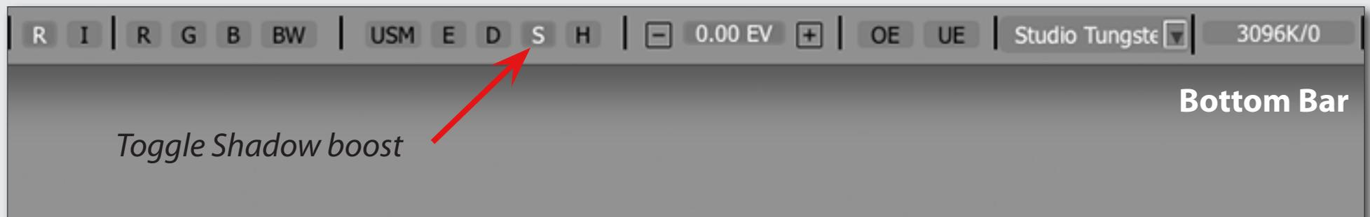
**Highlight Inspection** mode does the “opposite” of the **Shadow Boost** mode: the brightness of the shadows and midtones is decreased, thus the image looks darker; the contrast in the highlights is increased; white balance can be “canceled” by setting it to UniWB. As result it allows to evaluate details in highlights and inspect which channels are clipped (if any) and where.
